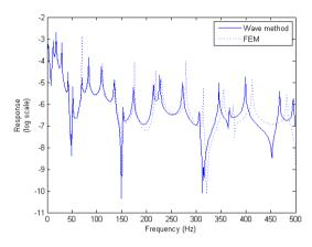
**Figure 9.** Response amplitude at x with force applied at Y for  $\Theta$ =35<sup>0</sup> frame
