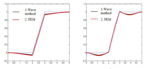
**Figure 6**. Comparison of first two modes shapes of  $\Theta$ =45<sup>0</sup> frame. The unreformed shape is shown as dotted line.
