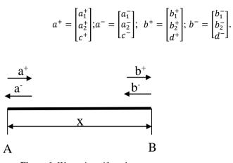
Figure 1. Waves in uniform beam.
