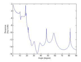
**Figure 8.** Response amplitude at x plotted as a function of  $\theta$  at frequency=200 Hz
