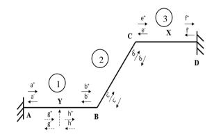
Figure 5. Waves in angular frame
