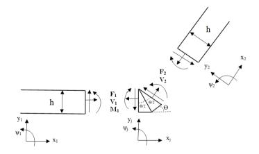
Figure 2. Free body diagram of angular joint.
