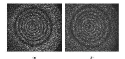
Fig. 4. Speckle correlation fringes with spatial phase shift: (a)  $-90^{0}$  and (b)  $0^{0}$
