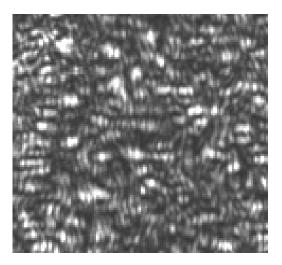
Fig. 3. Magnified portion of the speckle pattern with double aperture arrangement revealing the spatial carrier fringe
