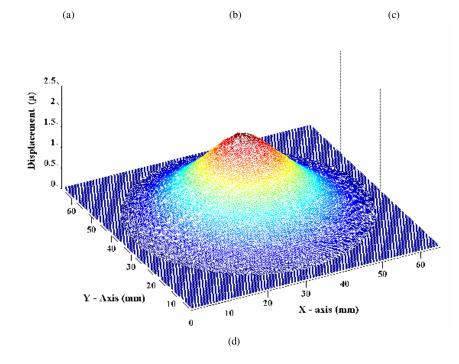
Fig. 5. Out-of-plane displacement measurement: (a) raw and (b) filtered phase maps, (c) unwrapped 2D and (d) 3D plots
