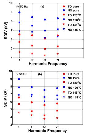
Figure 7. Variation in SDIV of OIP materials thermally aged in transformer oil and titania nanofluid under harmonic AC voltage with different THDs. (a) 4% THD and (b) 40% THD's Frequency Domain Analysis of UHF Signals
