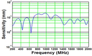
Figure 3. Frequency response of UHF sensor
