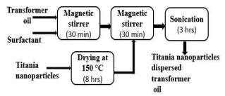
Figure 4. Preparation procedure of titania nanofluid with transformer oil as base
