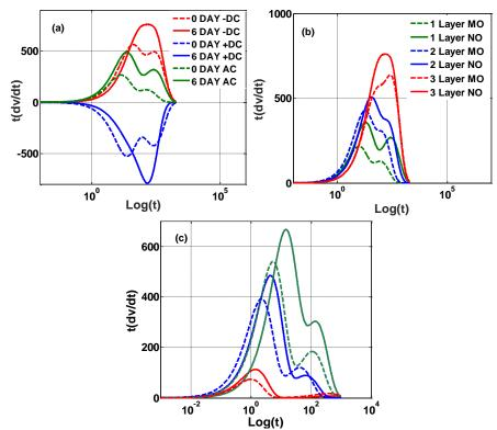
Figure 10. Variation tdV/dt curve of charge decay curve obtained under AC and DC voltage (a) AC and DC voltage profiles of virgin OIPs and thermally aged at 120 C, (b) layers for transformer OIPs and titanaia nanoparticles dispersed OIP materials of virgin material, and (c) with thermal aged material with three layers
