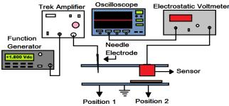
Figure 2. Experimental setup for charge accumulation
