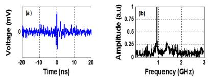
Figure 8. Typical (a) UHF signal formed due to surface discharge activity with titania nanofluid OIP material and (b) its corresponding FFT
