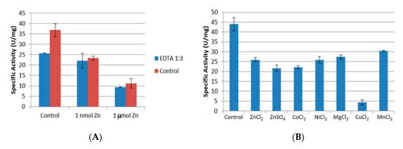
**Figure 3.** Effect of  $Zn^{2+}$  and other divalent metals on activity of CpCR. (**A**) Effect of  $Zn^{2+}$  (ZnSO<sub>4</sub>) on CpCR activity at various concentrations; (**B**) Specific activity of CpCR influenced by various divalent metal ions.
