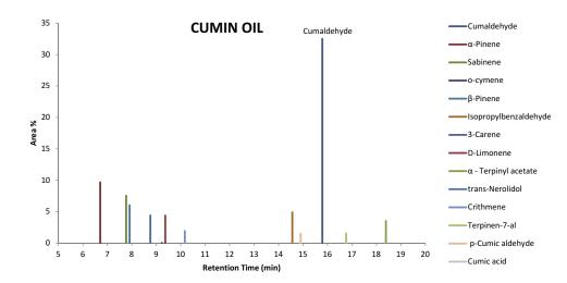
Figure I Gas Chromatography-Mass Spectroscopy of cumin essential oil extract.
