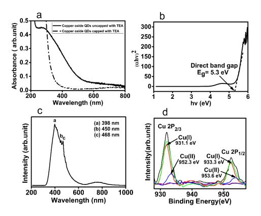
**Figure 2.** (a) UV–Vis absorbance spectra of uncapped and TEA capped copper oxide QDs, (b) Tauc plot for copper oxide QDs, (c) PL spectrum of copper oxide QDs using Xenon lamp of 200 nm as excitation, (d) smoothed and curve fitted XPS spectra of copper oxide QDs; 2p peak deconvolution is done with Lorentzian function. The spectrum obtained indicates that Cu exists in mixed valence state in this material.
