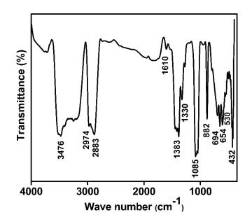
Figure 4. FT-IR spectrum of copper oxide QDs
