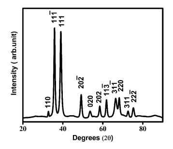
**Figure 1.** XRD pattern of CuO nucleated using higher concentration of precursors (30 mM Cu(OAc)<sub>2</sub>.2H<sub>2</sub>O and 180 mM NaOH) exhibiting monoclinic phase (Space group: C 2/c,#15).
