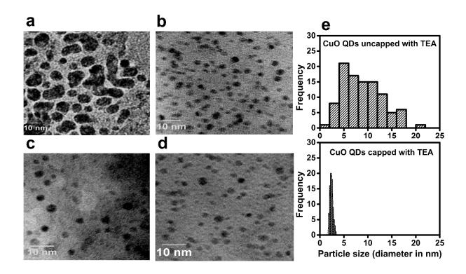
**Figure 3**. TEM images of (a) uncapped copper oxide QDs and (b) capped copper oxide QDs (c) TEM images of digestively ripened copper oxide QDs that are 120 days old. It may be noted from (a) that without capping particle coalescence is a concern. (d) TEM images of digestively ripened copper oxide QDs that are 1 year old. (e) Shows particle size distribution of copper oxide QD before and after digestive ripening.
