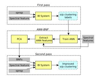
Figure 1: Block diagram of a two-pass IB based speaker diarization system. The first pass is the conventional IB system whose output is used to train an ANN with the speaker labels obtained. The bottleneck features from the ANN are then used in the second pass independently or complementary to the spectral features.
