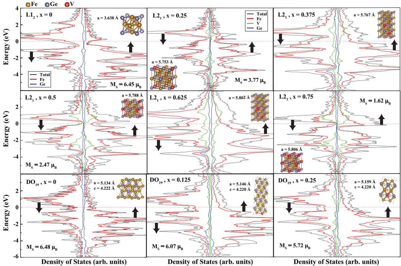
**Figure 13:** (color online) The DOS and PDOS of the lowest energy structure at specific concentration ratios for  $L2_1$ ,  $DO_{19}$ , and  $L1_2$ . The black arrows depict the spin up and spin down contributions and the red dotted line represents the Fermi level. The figure insets include the optimised structures, magnetic moment values and average lattice constants.
