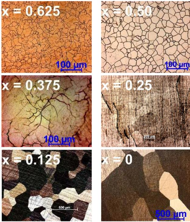
**Figure 1:** (colour online) Optical micrograph of  $\text{Fe}_{3-x}\text{V}_x\text{Ge}$  ( $0 \leq x \leq 1$ ) heat treated at  $950^\circ\text{C}$  for 7 days showing the grain structures. The samples were etched for 25 seconds using the Adler etchant.
