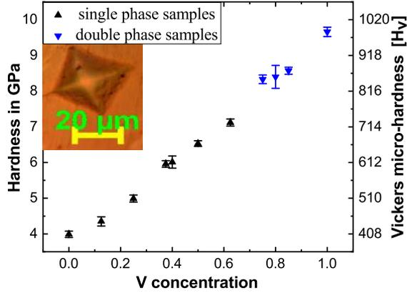
**Figure 10:** (color online) Vickers hardness versus V concentration in  $\text{Fe}_{3-x}\text{V}_x\text{Ge}$  with imprint of the indenter with radial cracks for  $x = 0$  [top left]. The black data points represent the single phase compositions.
