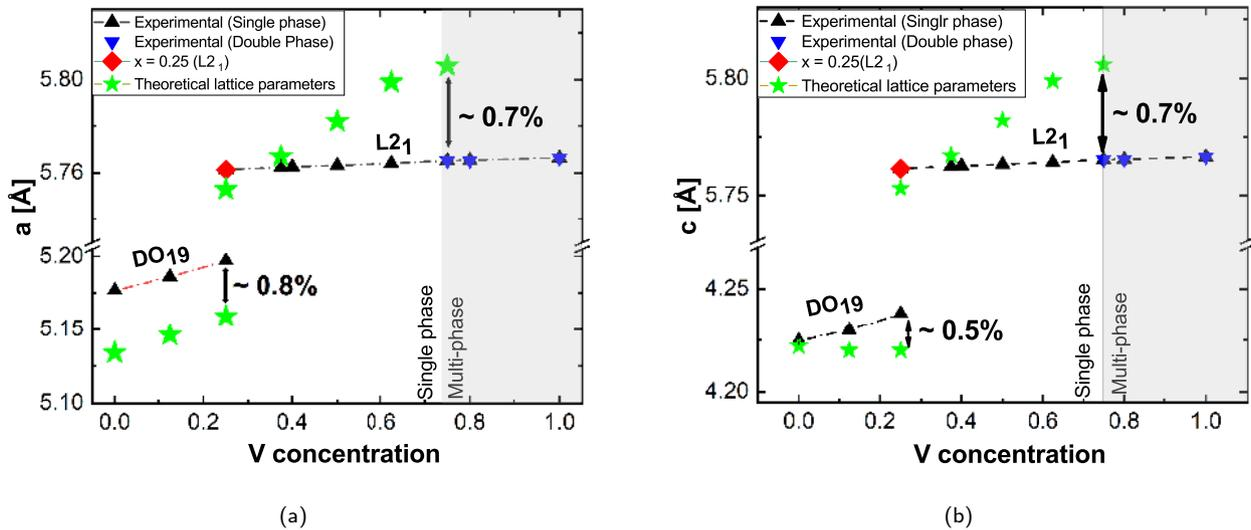
**Figure 12:** (color online) Comparison plot between experimentally extracted lattice parameters and theoretical values from First-principles calculations of  $\text{Fe}_{3-x}\text{V}_x\text{Ge}$  (a)  $a$  versus V concentration, and (b)  $c$  versus V concentration.
