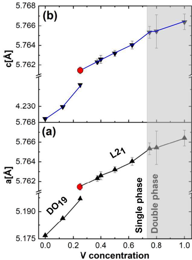
**Figure 6:** (color online) Variation of lattice parameters of  $\text{Fe}_{3-x}\text{V}_x\text{Ge}$  annealed at  $950^\circ\text{C}$  for 7 days (except the red data point representing  $x = 0.25$  annealed at  $650^\circ\text{C}$  for 25 days) (a)  $a$  versus  $V$  concentration, and (b)  $c$  versus  $V$  concentration. The shaded region represents multiphase region.
