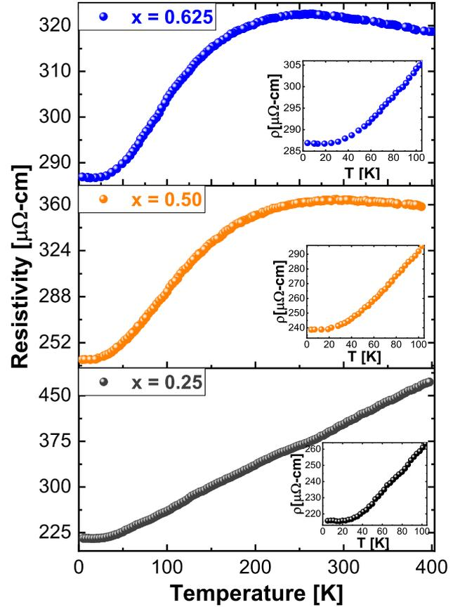
**Figure 9:** (color online) Temperature dependence of electrical resistivity in  $\text{Fe}_{3-x}\text{V}_x\text{Ge}$  ( $x = 0.25, 0.50$ , and  $0.625$ , all annealed at  $950^\circ\text{C}$  for 7 days respectively from bottom to top) in zero magnetic field.
