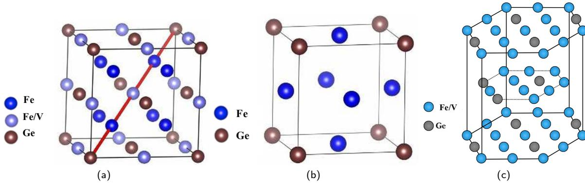
**Figure 5:** (color online) Various crystal structures (a)  $L2_1$ , (b)  $L1_2$ , and (c)  $DO_{19}$
