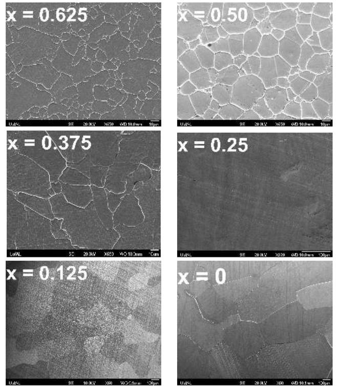
**Figure 2:** (color online) SEM micrograph of  $\text{Fe}_{3-x}\text{V}_x\text{Ge}$  ( $0 \leq x \leq 1$ ) heat treated at  $950^\circ\text{C}$  for 7 days showing the granular microstructure. The magnification of each micrograph is indicated at the bottom, like  $\times 650$  for  $x = 0.50$ .
