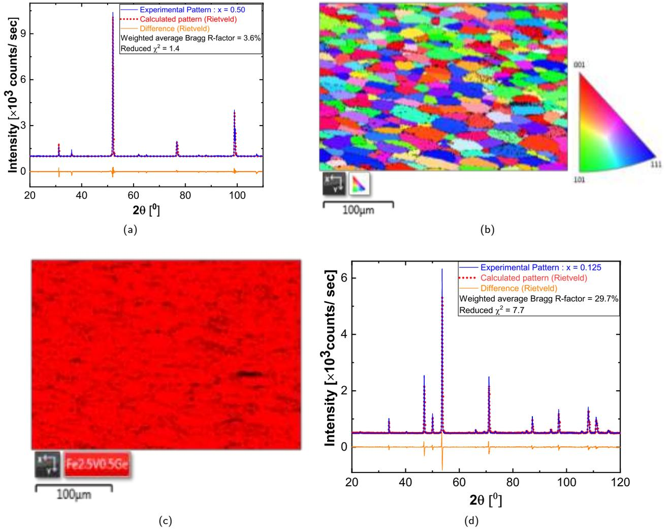
**Figure 4:** (color online) (a) The Rietveld refinement of XRD pattern showing a signature of good fit with the proposed crystal model  $L2_1$  (b) IPF color map (c) The corresponding EBSD phase color map of the same area of  $\text{Fe}_{2.50}\text{V}_{0.50}\text{Ge}$  in SEM (d) The Rietveld refinement of XRD pattern for  $\text{Fe}_{2.875}\text{V}_{0.125}\text{Ge}$  with the proposed  $\text{DO}_{19}$  crystal structure.
