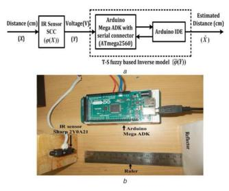
Fig. 8 *Real-time environment of IR sensor* (a) Schematic representation of the experimental environment, (b) Experimental setup for distance measurement
