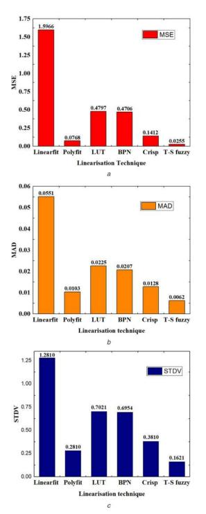
Fig. 11 Graphical error analysis of IR sensor using (a) MSE, (b) MAD, (c) STDV
