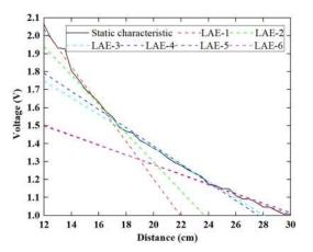
Fig. 9 IR sensor static characteristic
