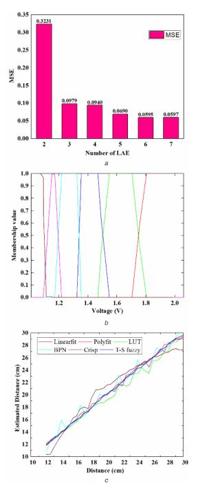
Fig. 10 Membership function and linearity analysis (a) MSE for the number of LAEs, (b) Membership function for IR sensor, (c) Linearity analysis of applied LT
