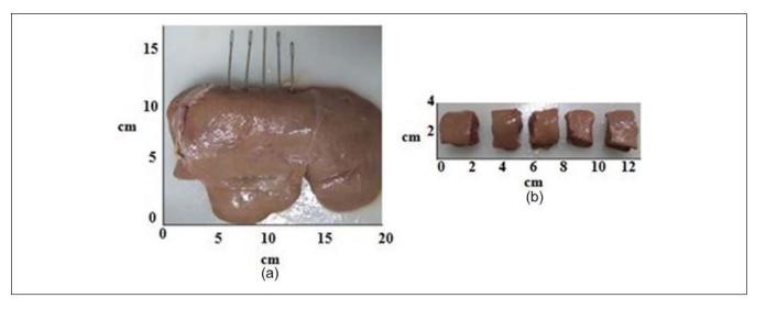
**Figure 4.** Image showing (a) the liver sample with needle insertions, which acts as a marker to identify the corresponding imaging planes and (b) the samples cut out from the liver for UTM testing. UTM = Universal Testing Machine.
