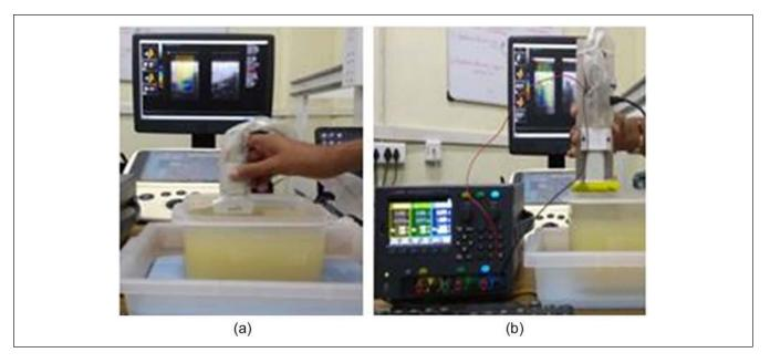
**Figure 3.** A photograph of the actual elastography data acquisition set up using Sonix Touch  $Q^+$  ultrasound scanner during (a) freehand compression and (b) handheld device compression.
