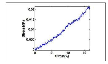
**Figure 6.** The plot of the stress-strain loading curve for one liver sample. The linear region is fixed at the initial portion (5% of strain), and Young's modulus was calculated as the slope of this linear portion using the least square fit.
