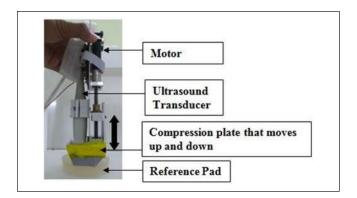
**Figure 2.** Photo of the handheld controlled compression setup (side view) along with reference pad.
