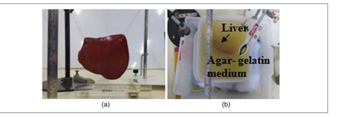
Figure 1. Photos showing (a) ex vivo liver suspended by stitching thread and held in place before agar-gelatin phantom solution is poured to surround it and (b) top view of the final liver-embedded Phantom.
