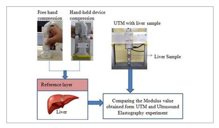
**Figure 5.** A schematic representation of the process for comparing the measurements obtained from quasi-static elastography (freehand and handheld device compression) integrated with the reference layer to that of UTM measurements. UTM = Universal Testing Machine.
