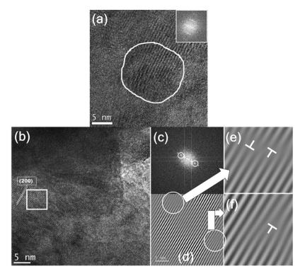
**Figure 3.** (a) HR-TEM image showing a nanocrystallite in 5 h BM alloy. The inset confirms the single crystal nature of the crystallite, (b) (200) plane observed in 5 h BM alloy, (c) The FFT from the region selected in (b) showing the SADP from the region, (d) The inverse FFT image from the selected points in (c) showing lattice fringes, (e,f) dislocations observed in the lattice corresponding to the regions indicated in (d).
