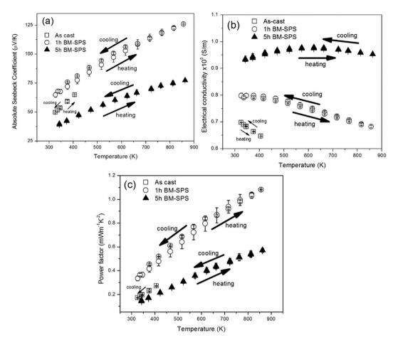
**Figure 4.** Variation of (a) Seebeck coefficient, (b) electrical conductivity and (c) power factor as a function of temperature for as-cast, 1 h BM-SPS and 5 h BM-SPS samples (heating and cooling cycles). Each data point is an average of 3 measurements. The error bars are indicated.
