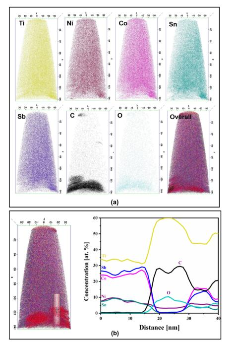
**Figure 7.** APT study on the 5 h BM-SPS alloy showing (**a**) elemental mapping to be devoid of segregation, (**b**) composition profile showing uniform composition across the cylinder.
