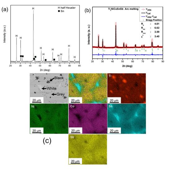
**Figure 1.** (a) XRD pattern, (b) Rietveld pattern of the VAM  $Ti_2NiCoSnSb$  alloy and (c) EDS Elemental mapping of the cast alloy confirming the presence of 3 phases.
