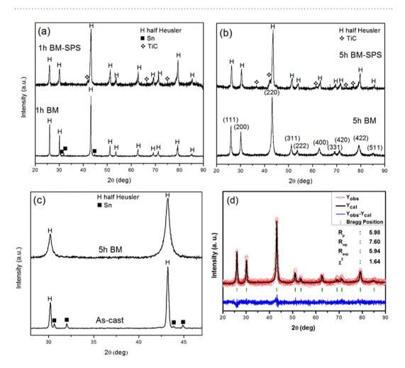
**Figure 2.** XRD pattern of (**a**) 1 h BM and 1 h BM-SPS alloy, (**b**) 5 h BM and 5 h BM-SPS alloy, (**c**) zoomed in region of 5 h BM alloy showing absence of Sn peaks, (**d**) Rietveld refinement pattern of the 5 h BM alloy.
