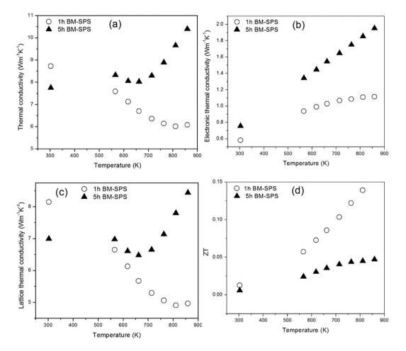
Figure 5. (a) Total thermal conductivity, (b) electronic thermal conductivity, (d) lattice thermal conductivity and (d) thermoelectric figure of merit (ZT) of  $Ti_2NiCoSnSb$  alloy.
