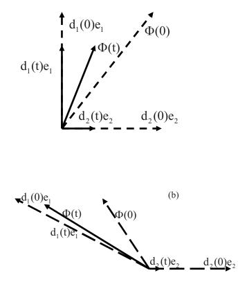
FIG. 1. (a) Monotonic decay of a normal system; (b) transient growth of a non-normal system. The initial state is  $\Phi(0)=d_1(0)e_1+d_2(0)e_2$ , and the final state is  $\Phi(t)=d_1(t)e_1+d_2(t)e_2$ . The dashed lines denote the vectors at time t=0 and the solid lines denote the vector at some time t.
