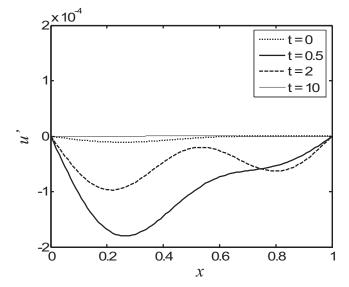
FIG. 8. Spatial variation of the acoustic velocity at various instants of time. The initial condition is chosen to be the optimum initial condition which yields the maximum growth factor.  $L_w$ =2.0 m,  $\tau$ =0.1 $\pi$ ,  $\lambda$ =0.0328 W/m K,  $C_v$ =719 J/kg K,  $\bar{\rho}$ =1.205 kg/m<sup>3</sup>,  $c_0$ =401.2 m/s,  $\bar{u}$ =0.6 m/s, and  $T_w$ =900 K.
