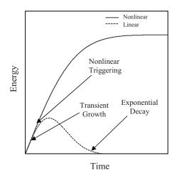
FIG. 2. Schematic of linear and nonlinear evolutions of the acoustic energy  $\left[\frac{1}{2}p'^2 + \frac{1}{2}(\gamma M u')^2\right]$ .
