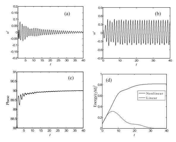
FIG. 4. Evolution of nondimensional acoustic velocity when the initial conditions are (a)  $\eta_1(0)=0.15$  and (b)  $\eta_1(0)=0.2$ ,  $x_f=0.29$ ,  $c_0=399.6$  m/s,  $L_w$ = 3.6 m,  $\bar{u}=0.5$  m/s,  $\bar{\rho}=1.205$  kg/m<sup>3</sup>,  $T_w=1000$  K,  $C_v=719$  J/kg K, and  $\lambda=0.0328$  W/m K. (c) Evolution of phase and (d) linear and nonlinear evolutions of the acoustic energy when the initial condition is  $\eta_1(0)=0.2$ .
