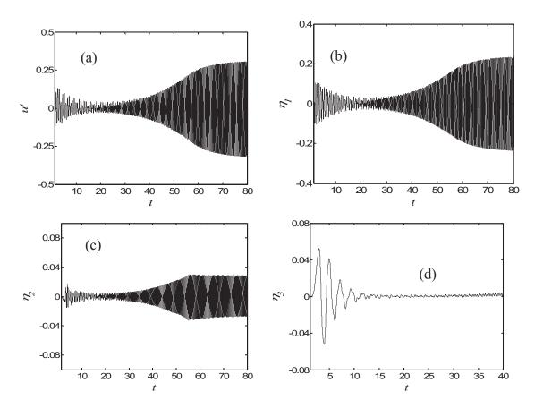
FIG. 5. (a) Nondimensional evolution of acoustic velocity when the initial condition is  $\eta_1(0)=0.18$ ; [(b)–(d)] evolution of the acoustic velocity projected onto the various Galerkin modes.  $L_w=3.6$  m,  $\lambda=0.0328$  W/m K,  $C_v=719$  J/kg K,  $\bar{\rho}=1.205$  kg/m<sup>3</sup>,  $\bar{u}=0.5$  m/s,  $T_w=1000$  K,  $\tau=0.45\pi$ ,  $x_f=0.29$ , and  $c_0=399.6$  m/s.
