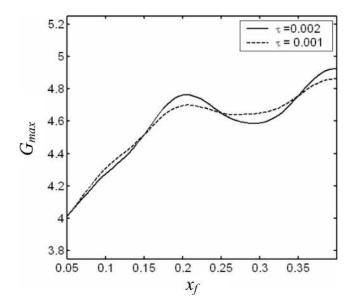
FIG. 7. Variation of maximum growth factor with heating element location for different values of time lag.  $L_w$ =2.0 m,  $\lambda$ =0.0328 W/m K,  $C_v$ =719 J/kg K,  $\bar{p}$ =1.205 kg/m<sup>3</sup>,  $c_0$ =401.2 m/s,  $\bar{u}$ =0.5 m/s, and  $T_w$ =1000 K.
