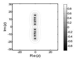
FIG. 9. Pseudospectra of a Rijke tube in which the heater is located at  $x_f$  =0.18. The time lag was chosen as  $\tau$ =0.1 $\pi$ .  $\lambda$ =0.0328 W/m K,  $C_v$ =719 J/kg K,  $c_0$ =399.6 m/s,  $\bar{\rho}$ =1.205 kg/m<sup>3</sup>,  $L_w$ =2.0 m,  $T_w$ =1000 K, and  $\bar{u}$ =0.5 m/s.
