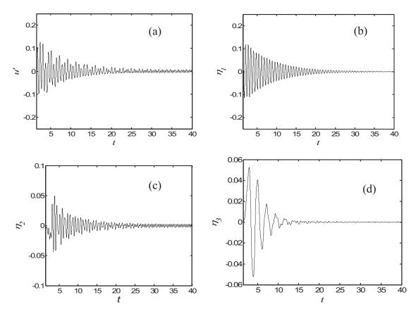
FIG. 6. (a) Linear evolution of acoustic velocity when the initial condition is  $\eta_1(0)=0.18$ ; [(b)–(d)] evolution of the acoustic velocity projected onto the various Galerkin modes. The conditions are the same as those of Fig. 5.
