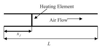
FIG. 3. Schematic of the horizontal Rijke tube setup.
