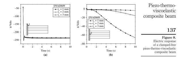
to propagate to the sensor layer and also some amount of the heat dissipation takes place in viscoelastic layer hence only piezoelectric effect is dominant.
