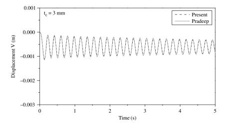
**Figure 5.** Validation with isotropic piezo-thermo-viscoelastic clamped free beam with 3 mm core thickness
