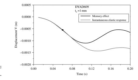
Figure 7. Effect of viscoelastic memory on mechanical response of a piezo-thermo-viscoelastic composite beam in zoomed view
