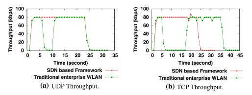
Figure. 4. Throughput when the sender application runs on the remote host.
