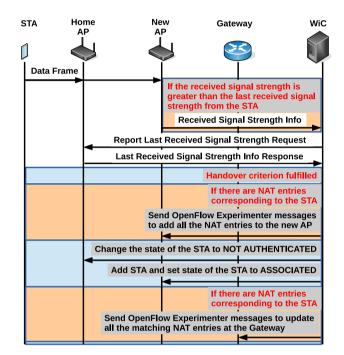
Figure. 2. Handover process for NAT operation mode.
