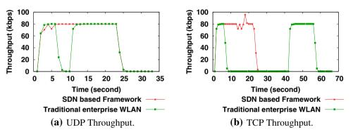
Figure. 3. Throughput when the sender application runs on the mobile node or station.
