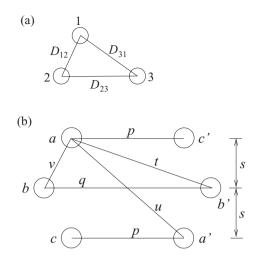
Fig. 3 Single circuit and double circuit lines. (a) Single circuit line; (b) double circuit line.
