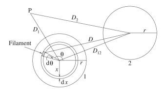
Fig. 1 Cross-section of two parallel straight conductors.
