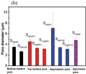
Fig. 4 Average porosity of the film (a) and average pore diameter (b) of the film surface in contact with the glass substrate obtained under different experimental conditions.
