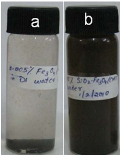
FIG. 5. (Color online) Photograph of (a) \text{Fe}_3\text{O}_4/\text{MWNT} and (b) \text{Fe}_3\text{O}_4@/\text{SiO}_2/\text{MWNT} nanofluid (in DI water) without surfactant. The photograph was taken after one week of the synthesis.
