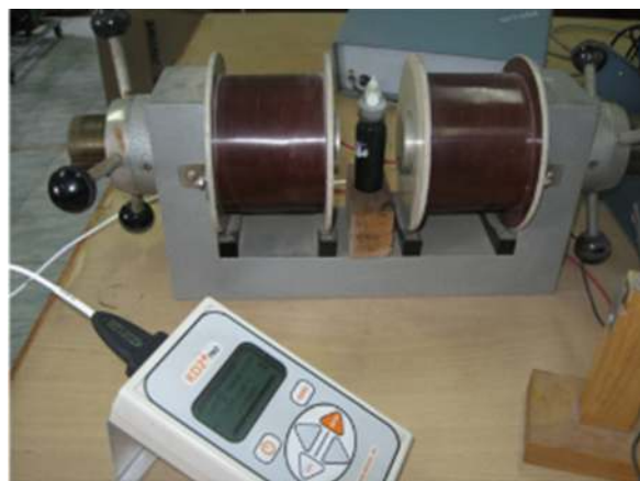
FIG. 1. (Color online) Experimental setup used for the measurement of the thermal conductivity of the magnetic nanofluid in the presence of magnetic field.
