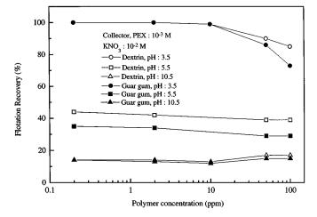
**FIG. 8.** Effect of dextrin and guar gum concentration on the flotation recovery of pyrite.
