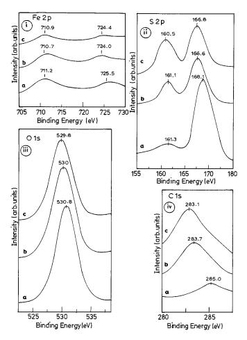
**FIG. 12.** X-ray photoelectron spectra of pyrite in the absence and presence of dextrin and guar gum for (i) Fe 2p, (ii) S 2p, (iii) O 1s, and (iv) C 1s regions.
