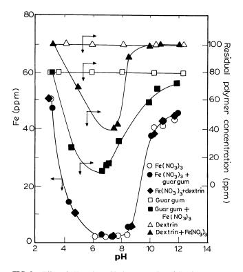
**FIG. 9.** Effect of pH on the residual concentration of dextrin or guar gum and iron.
