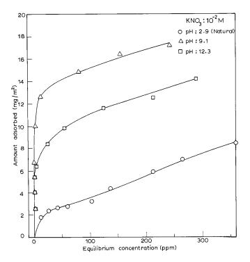
FIG. 4. Adsorption isotherms of guar gum onto pyrite.
