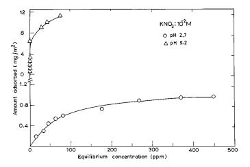
FIG. 3. Adsorption isotherms of dextrin onto pyrite.
