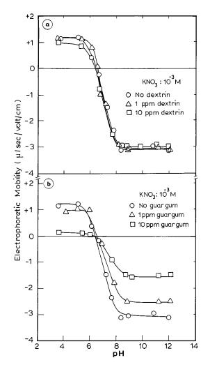
**FIG. 6.** Electrophoretic mobility of pyrite as a function of pH in the absence and presence of different concentrations of (a) dextrin and (b) guar gum.
