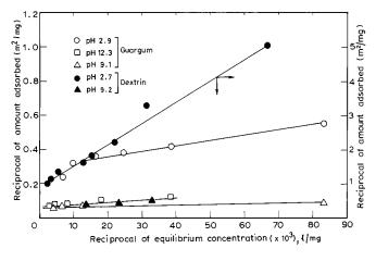
**FIG. 5.** Plot of reciprocal of adsorption density versus reciprocal of equilibrium concentration of dextrin and guar gum.
