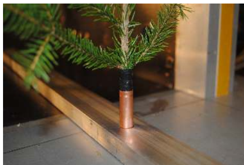
Figure B.18: Branch inserted in rig (Paper 4).
