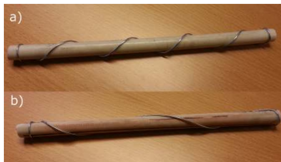
Figure B.27: Helical steel wire with a pitch of a) 8D and b) 4D, added to the circular cylinder.
