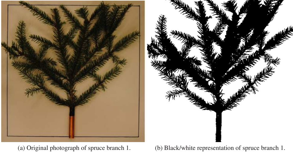
Figure B.19: Photograph analysis of blockage ratio (Paper 4).
