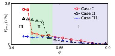
Figure 3. Variation of the root mean square of the unsteady pressure fluctuations,  $P_{rms}$ , as a function of the equivalence ratio  $\phi$  for case I (-  $\Box$  -), case II (-  $\triangle$  -) and case III (-+-).
