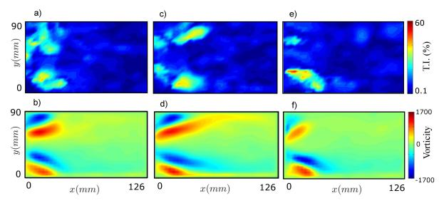
Figure 2. Time-averaged turbulence intensity fields - T.I. (a, c, e) and the corresponding time-averaged vorticity fields (b, d, f) obtained from the cold flow experiments. (a, b) correspond to case I, (c, d) refer to case II and (e, f) correspond to case III. x refers to the distance from the dump plane while y refers to the distance in the vertical direction.
