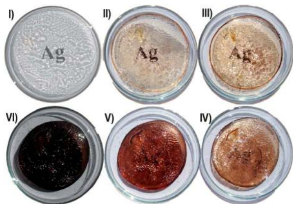
Fig. 1 (I) Photograph of the polymerized form of acrylamide gel along with oligomeric Ag(I)SG, taken in a Petri dish. (II), (III), (IV), (V) and (VI) are photographs corresponding to the exposure to sunlight at different time intervals of 5 min, 30 min, 1 h, 3 h, and 6 h, respectively. The Petri dish was placed on white paper with the label, 'Ag' printed on it. Note the change in transparency from (I) to (VI). The gel shrinks upon irradiation as water evaporates and the dry gel is detached from the Petri dish.
