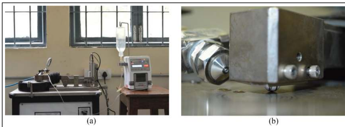
Figure 4. Setup for measuring the coefficient of friction, \mu for different CFs: (a) general setup with flow control infusion pump and (b) positioning of nozzle and ball.
