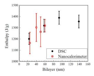
FIG. 4. Plot of heats of reaction measured using Ni:Al bilayer samples and the nanocalorimeter and Ni:Al multilayer samples and a conventional DSC. Error bars represent the mean plus and minus one standard deviation. For the DSC measurements N = 4, with the same heating rate. For the nanocalorimeter N = 3, with different heating rates.
