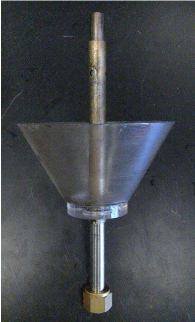
Fig. A-1.5: Burner with 60° Cone Feeder
