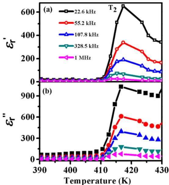
FIG. 3. Temperature variation of (a)  $\epsilon_r'$  and (b)  $\epsilon_r''$  for the DIPAB film (heat treated at 428 K-monoclinic- $P2_1$ ) at various frequencies.
