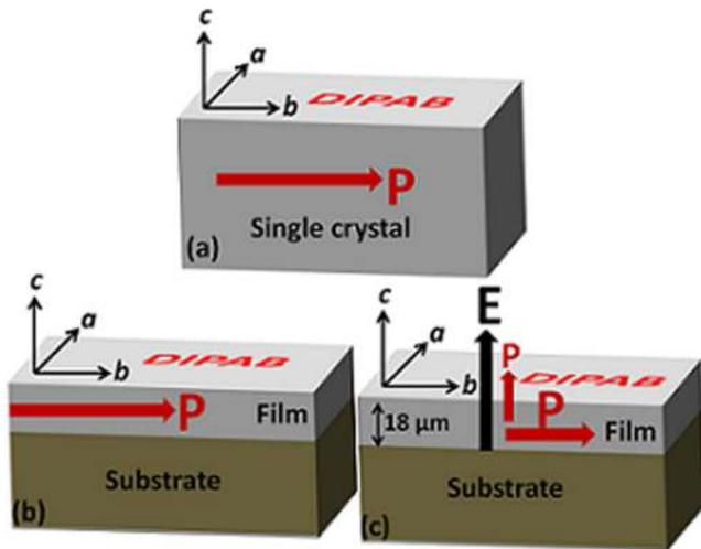
FIG. 8. A schematic representation of polarization direction in DIPAB: (a) single crystal, (b)  $c$ -axis oriented thick film in the absence of electric field, and (c)  $c$ -axis oriented thick film in the presence of electric field.
