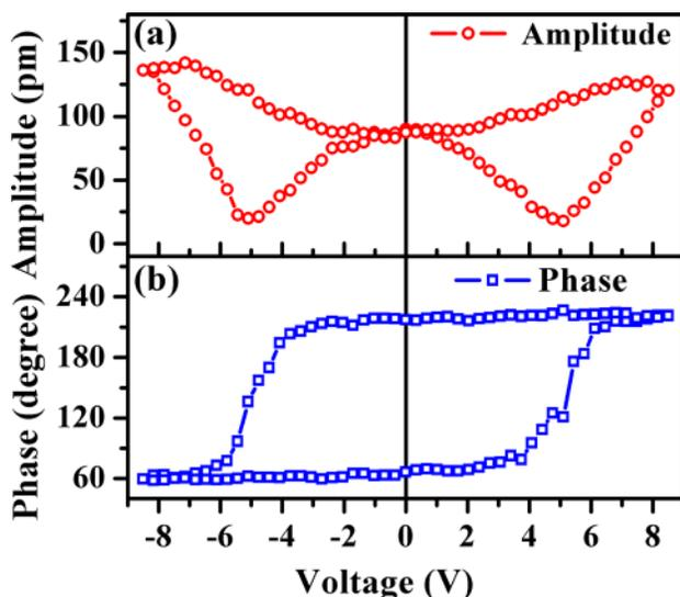
FIG. 6. The piezoresponse spectroscopic (a) amplitude and (b) phase response of the DIPAB film.
