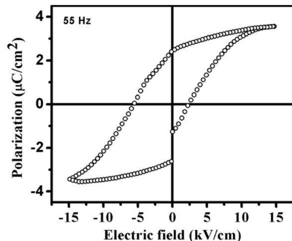
FIG. 7. The polarization versus electric field measured at 300 K for DIPAB film.
