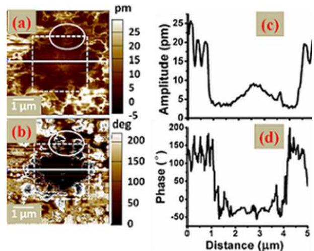
FIG. 5. The PFM (a) amplitude and (b) phase images of the DIPAB film (after writing). The corresponding line profiles are shown in (c) and (d).
