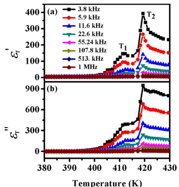
FIG. 2. Temperature variation of (a)  $\epsilon_r'$  and (b)  $\epsilon_r''$  for the DIPAB film (cured at 300 K-orthorhombic- $P2_12_12_1$ ) at various frequencies.
