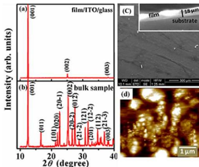
FIG. 1. X-ray diffraction pattern of DIPAB (a) film on the ITO/glass substrate and (b) bulk sample. (c) The SEM image of the DIPAB film surface and (d) PFM topographic image of the DIPAB film.
