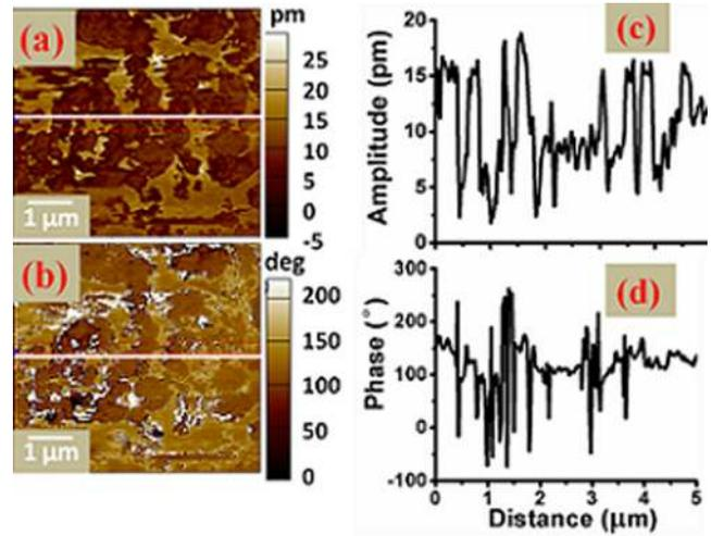
FIG. 4. The PFM (a) amplitude and (b) phase images of the DIPAB film (before writing). The corresponding line profiles are shown in (c) and (d).
