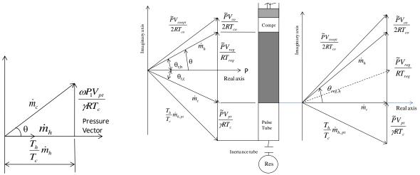
Figure 2. Phasor representation for flow through the Pulse tube.
