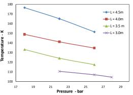
**Figure 10.**  $\phi$  1.76 mm Inertance tube Temperature variation with Charge Pressure.
