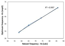
**Figure 9.**  $\phi$  1.76 mm Inertance tube Correlation between Calc and Opt frequency.
