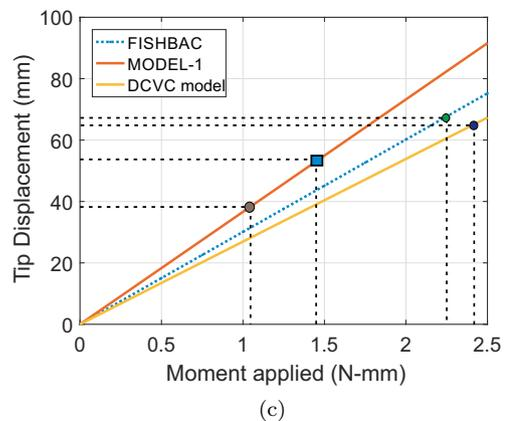
Fig. 5. Mechanical study under external moment load for various configuration. (a) Stress developed in the skin (b) Stress developed in the corrugated sheet (c) Tip displacement.
