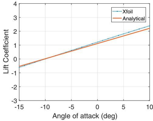
Fig. 8. Comparison of analytical lift coefficient with that of Xfoil results. The analysis is carried out assuming thin airfoil theory.
