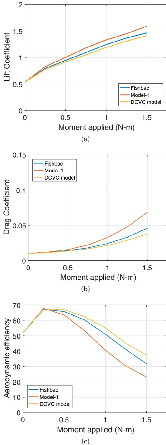
Fig. 10. Variation of aerodynamic coefficients with tendon moment : (a) Lift coefficient (b) Drag coefficient and (c) Lift-to-Drag ratio.
