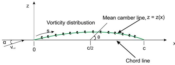
Fig. 7. Placement of the Vortex sheet on camber line.
