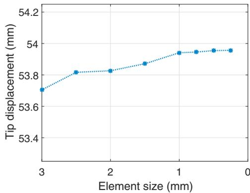
Fig. 4. Convergence study for DCVC model. Tip displacement plotted against element size.
