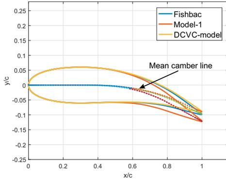
Fig. 6. Deformed structural shapes of all configurations with tendon moment ( $M = 1 \text{ N-m}$ ).
