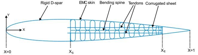
Fig. 2. Morphing wing composed of double corrugated structure with trailing edge morphing section and bending spine (This is referred to as DCVC in the text).
