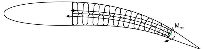
Fig. 3. Representation of tendon and trailing edge bending.
