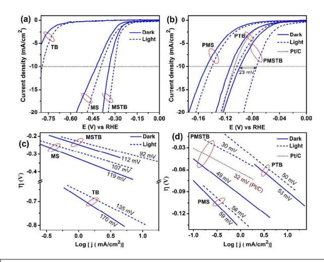
Fig. 8: Polarization curves of the hydrogen evolution reaction (HER) in dark and light conditions in (a) pristine  $TiO_2(B)$ ,  $MoS_2$  and  $MoS_2/TiO_2(B)$  HS, (b)  $Pt@MoS_2$ ,  $Pt@TiO_2$  and  $Pt@MoS_2/TiO_2$  HSs. (c, d) Tafel plots of different working electrodes derived from their LSV curves shown in (a,b), respectively. Polarization curve and the corresponding Tafel plot for Pt/C electrode are also shown in (b, d), respectively.
