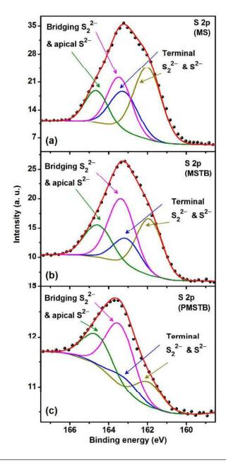
Fig. 5: S 2p core level XPS spectra for (a) MS, (b) MSTB and (c) PMSTB, fitted with the Shirley baseline. The symbols represent the experimental data and the solid lines correspond to the Gaussian fits. Identity of each fitted peak is denoted with corresponding charge states in the respective cases.
