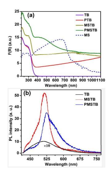
Fig. 7: (a) Kubelka–Munk plot, F(R), for different samples derived from the diffuse reflectance spectra. (b) PL spectra of TiO<sub>2</sub> and its HSs measured with 405 nm laser excitation. The PL spectrum of TB is shown in magnified scale to enable comparison.
