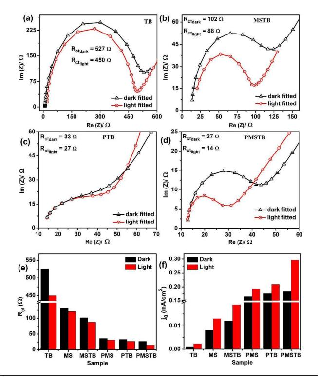
Fig. 9: Nyquist plots of (a) pristine  $TiO_2(B)$ , (b)  $MoS_2/TiO_2$ , (c)  $Pt@TiO_2$  and (d)  $Pt@MoS_2/TiO_2$  HSs, under dark and light conditions. Note that the points represent experimental data, while the solid lines are simulation using the Randle's circuit to estimate the characteristic charge-transfer resistance ( $R_{ct}$ ). (e, f)  $R_{ct}$  and  $j_0$  values, respectively, of various electrodes in dark and light conditions.
