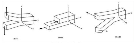
Fig. 1. Basic modes of delamination
