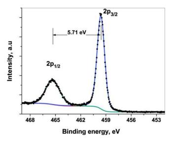
FIG. 5. (Color online) XPS Ti2p spectrum of nanocrystalline anatase having crystallite size 7 nm.
