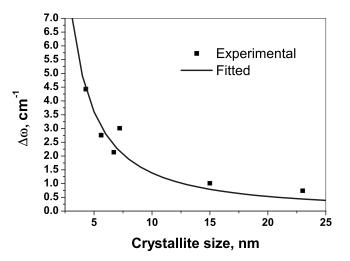
FIG. 4. Shift in 144 cm<sup>-1</sup> peak in Raman spectra of nanocrystalline anatase powders.
