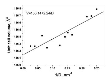
FIG. 3. Crystallite size dependence of unit cell volume of anatase.
