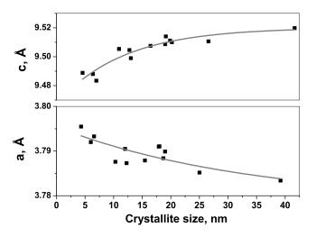
FIG. 1. Effect of crystallite size on the lattice parameters a and c of anatase.
