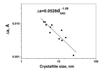
FIG. 2. Crystallite size dependency of change in the lattice parameter, a.
