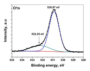
FIG. 6. (Color online) XPS O1s spectrum of nanocrystalline anatase having crystallite size 7 nm.
