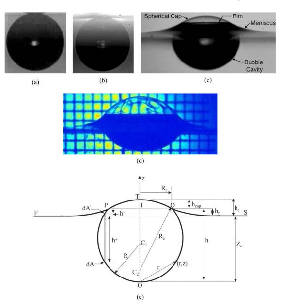
FIG. 1. [(a)–(d)] Side views of floating air bubbles at different Bond numbers. (a)  $R_e = 0.175$  mm,  $Bo_e = 0.004$ ; (b)  $R_e = 0.47$  mm,  $Bo_e = 0.03$ ; (c)  $R_e = 1.99$  mm,  $Bo_e = 0.5$ ; (d)  $R_e = 3.61$  mm,  $Bo_e = 2.46$ ; (e) schematic of a floating bubble with the present notation  $h_c = h_{cap} + h_r$ .
