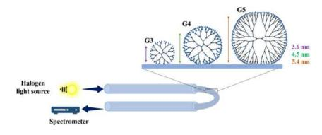
Figure 1. Schematic showing the experimental set-up with dendrimer-coated PMMA-POF coupled to a halogen light source and fiber optic spectrometer. Inset: PMMA surface modification with PAMAM dendrimer of different generations (G3, G4 and G5) and their dimensions explored in this study.
