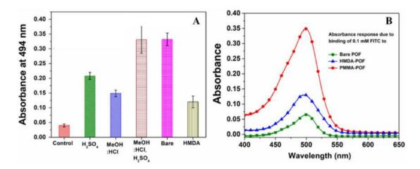
**Figure 2.** (A) Absorbance response due to FITC binding to (i) control (without G4 PAMAM dendrimer surface modification) and G4 PAMAM dendrimer-coated U-bent POF probes that are pre-treated with (ii) 1 M H2SO4, (iii) MeOH-HCl, (iv) their combination and (v) without any pre-treatment. (B) Absorbance response from U-bent POF probes due to FITC binding to bare (spheres), HMDA functionalized following an acid pre-treatment (triangles) and G4 PAMAM functionalized (squares) probes U-bent PMMA-POF.
