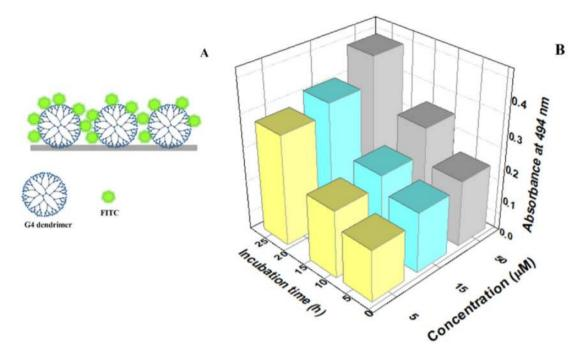
Figure 3. (A) Schematic representation of FITC binding to G4 PAMAM dendrimer on U-bent PMMA-POF probe surface and (B) saturated absorbance response at 494 nm of U-bent POF with varying incubation time and concentration of dendrimer solution (the probes were incubated in FITC solution of 0.1 mM concentration).
