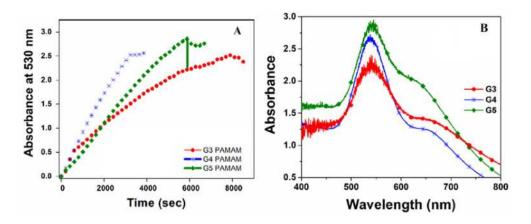
Figure 5. (A) Temporal response at 530 nm and (B) absorbance response obtained from U-bent POF probes functionalized with dendrimer of a different generation and thereafter, subjected to AuNP (OD 1.5).
