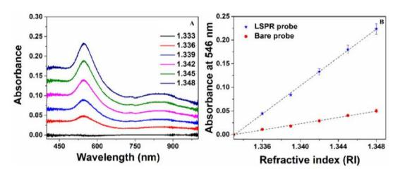
Figure 6. (A) Absorbance response and (B) RI sensitivity obtained from developed P-FOS subjected to sucrose solution of varying RI taking DI water as a reference.
