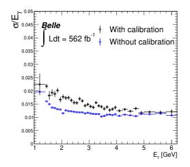
Figure 1. Energy resolution as a function of the reconstructed photon energy in the  $e^+e^- \rightarrow \mu^+\mu^-\gamma$  events. Black (Blue) points are the photon energy resolution with (without) the calibration applied. Error bars are the statistical uncertainties.
