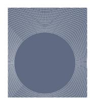
Fig. 3. closeup view of mesh around cylinder
