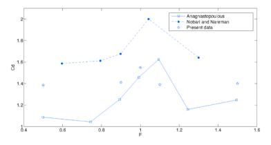
Fig. 6. Comparison of Drag coefficients versus forcing frequency (F) for an oscillating circular cylinder
