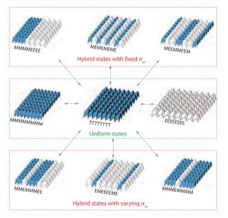
Fig. 6 Realizations of the Morph pattern with  $8 \times 8$  cells—the three uniform states and sample hybrid states. The double arrows indicate inter-transformability between states. *M*, *E*, *T* represent the strips in Miura mode, Eggbox mode, and Transition state, respectively. The parameter  $n_m$  is the number of strips in the Miura mode. The strips in the Eggbox mode are shown in white color.
