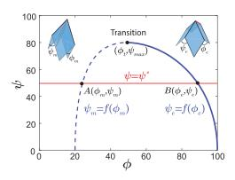
Fig. 2 Configuration path of a Morph unit cell in terms of the folding angles. The Miura mode cells are represented by point A and the Eggbox mode cells are represented by point B which lie on the dashed and solid curves, respectively.
