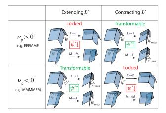
Fig. 9 Mode-locking and transformability of the hybrid states of the Morph pattern under deformation
