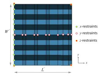
Fig. 10 Plan view of the hybrid Morph pattern with  $6 \times 6$  cells showing the displacement restraints imposed on the nodes (vertices) for the numerical simulations
