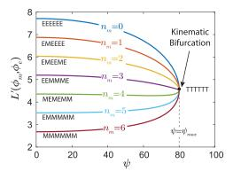
Fig. 7 Kinematic branches of the Morph pattern. *EEEEEE*, *MMMMMM*, *TTTTTT* are uniform states and the rest are hybrid states. The parameter  $n_m$  denotes the number of strips in the Miura mode. The panel geometry was chosen as  $\alpha = 60 \text{ deg}$ ,  $\beta =$ 40 deg, and a = 1.
