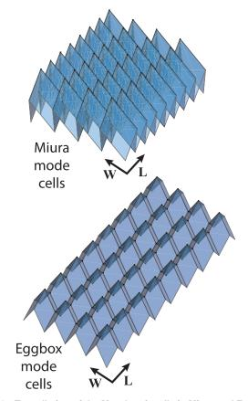
Fig. 4 Tessellation of the Morph unit cells in Miura and Eggbox modes to form uniform Morph patterns
