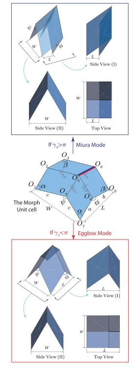
Fig. 1 The two characteristic modes of the Morph unit cell: Miura mode and Eggbox mode
