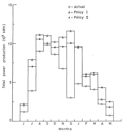
Fig. 4 Comparison of total power production monthwise.
