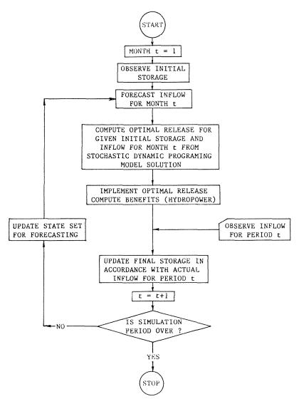
Fig. 2 Block diagram for real-time simulation.
