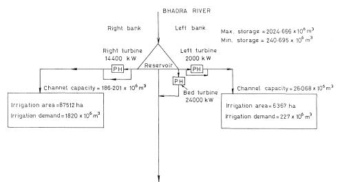
Fig. 1 Schematic diagram of Bhadra reservoir project.
