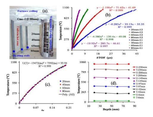
FIG. 4. (a) Shows the multiple-sensors of a helical waveguide at uniform temperature zone in the furnace. (b) The  $\delta$ TOF's of each notch sensors at various temperatures. (c)  $\epsilon_{u}$  vs Temperature for all notches representing the calibration curve. (d) Comparison of temperature measurement using ultrasonic waveguide method (solid) with thermocouple (hollow).
