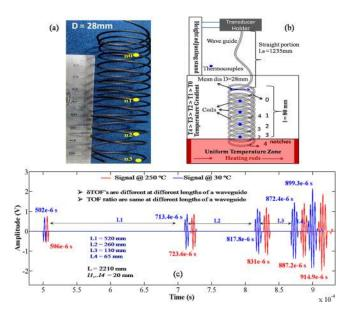
FIG. 3. (a) Photograph of Chromel helical waveguide with notches. (b) Schematic diagram of multiple notches (sensors) in a helical waveguide system with melter. (c) Reflected signals as received from the 4 notches and the end of the helical waveguide at different temperatures.
