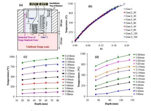
FIG. 5. (a) Multiple sensors of a helical waveguide at insulated region of the furnace. (b) Multiple sensors waveguide calibration from 160 mm depth of temperature gradients. (c) Ultrasonic and thermocouple measurements from different depths at different time instances using 80 mm free length of helical waveguide. (d) Ultrasonic and thermocouple measurements from different depths using 160 mm free length.
