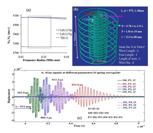
FIG. 2. (a) Dispersion curves (Phase velocity- $V_p$  and Group velocity- $V_g$ ) for a straight Chromel wire. (b) Helical waveguide dimensions at different parameters. (c) A-scan of the far end reflected signals obtained in pulse echo mode at different D, P, and *l* values listed in Table II.
