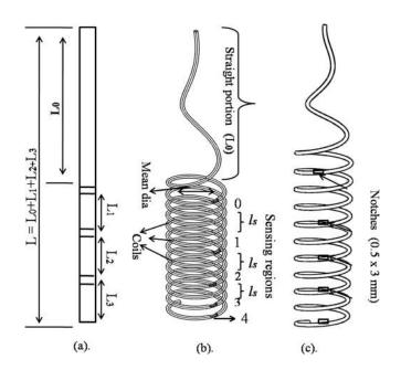
FIG. 1. Illustration of temperature gradient measurement concept in (a) straight waveguide, (b) and (c) Helical waveguides.
