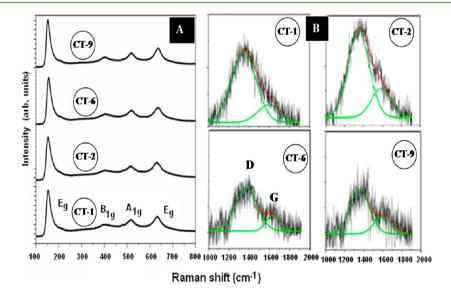
Figure 5. Raman profiles of the spherical (CT-1), distorted spherical (CT-2), hexagonal (CT-6), and rice grain (CT-9) shaped C-TiO<sub>2.</sub> (A) TiO<sub>2</sub> bands in the low frequency region; (B) D and G bands in the higher frequency region.
