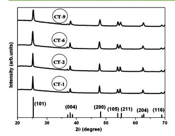
**Figure 4.** XRD profiles of the four different morphologies of C-TiO<sub>2</sub>. For comparison, XRD of bulk anatase TiO<sub>2</sub> is plotted in the bottom (ICPDS 89-4921).
