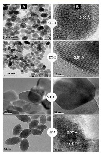
Figure 3. TEM images at (A) low and (B) high magnification of spherical (CT-1), distorted spherical (CT-2), hexagonal (CT-6), and rice grain (CT-9) shaped of  $C-TiO_2$  NCs.
