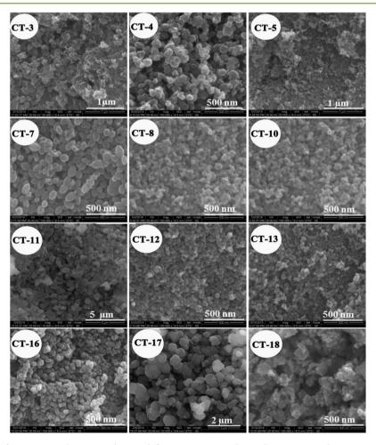
Figure 2. HRSEM images of C-TiO<sub>2</sub> samples prepared using different reaction conditions by microwave digestion technique.
