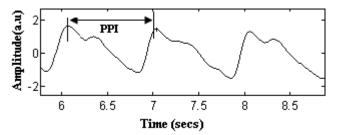
Fig. 1. Peak-to-Peak interval (PPI) in a typical PPG signal
