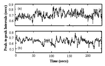
Fig. 3. Peak-to-Peak intervals (PPI) extracted from PPG signal in (a) Fasting state and (b) Postprandial state
