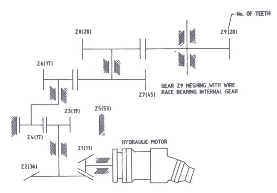
Figure 5. Kinematic diagram of armoured fighting vehicle's traverse gear box
