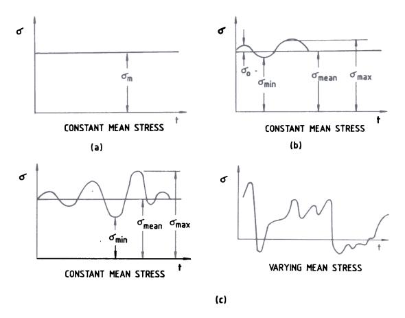
Figure 1. Classification of stress time history: (a) static stress, (l) periodically varying stress, and (c) irregularly varying stress
