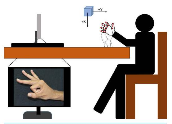
Figure 2 Experimental setup. Participants were seated in a height-adjustable chair. Placement of the transmitter was based on biomechanical standards (*Wu et al.*, 2005). The computer screen was placed approximately 1 m away from the participant. Image of posture was shown to the participant on the screen. Participants were asked to perform posture which is shown on the screen starting from the base posture.
