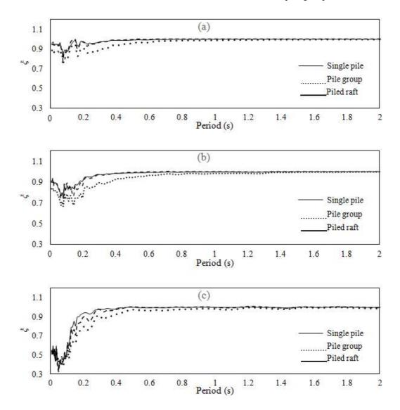
Figure 6. Spectral ratio for (a) Central Mexico 2017, (b) Ferndale 2014, and (c) Valparaiso 2017 ground motions
