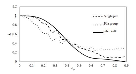
Figure 5. Transfer function in translation for the three foundation cases.
