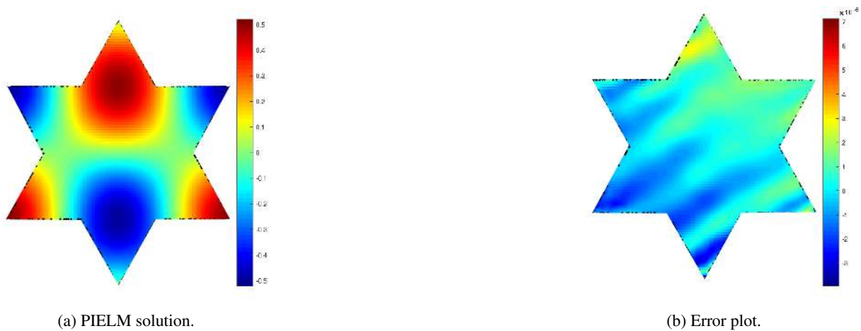
Figure 8: Solution and error for 2D steady advection equation on \Omega_1 .
