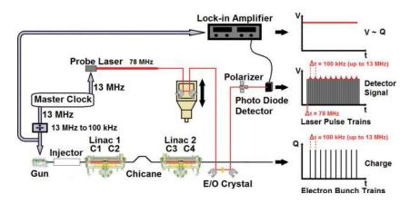
FIG. 1. Schematic of the phase and frequency locked electro-optic monitor concept employed in the pilot experiments at ELBE. The present set up allows to work at repetition rates between 100 kHz and 13 MHz in both, continuous wave (cw) and macro pulse (mp) mode of operation, respectively.
