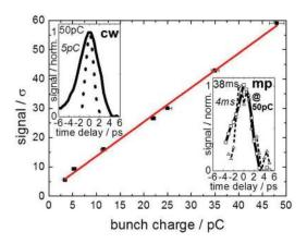
FIG. 2. EOS-signal in units of the standard deviation  $\sigma$  for different bunch charges utilizing 300 ms integration times. (*Inset top left*): Measurements at a bunch charge of 50 pC (solid) and 5 pC (dashed) in continous wave (cw) mode of operation. (*Inset bottom right*): Measurements in macro pulsed (mp) mode of operation at a charge of 50 pC, a repetition rate of 25 Hz (macro pulses)/100 kHz (micro pulses), and a macro pulse duration of 38 ms (squares) and 4 ms (triangles).
