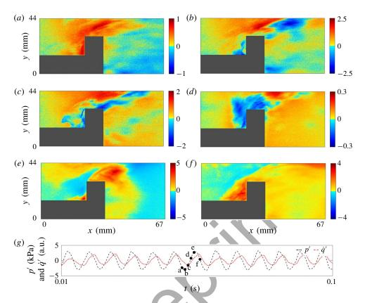
FIGURE 7. (Colour online) (a-f) Instantaneous fields of local acoustic power production  $p'\dot{Q}'(x, y, t)$  at different instants of time (t) during the occurrence of thermoacoustic instability for one periodic cycle. (g) Simultaneous p'(t) and  $\dot{q}'(t)$  (obtained from PMT). Here, we observe that the fields of  $p'\dot{Q}'(x, y, t)$  comprise of regions of coherent dynamics.
