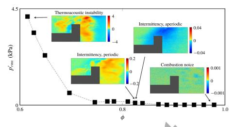
FIGURE 13. (Colour online) The variation in the  $p'_{rms}$  with respect to the equivalence ratio. The insets are instantaneous fields of local acoustic power production for the corresponding equivalence ratio. This figure shows the emergence of the self-organized coherent regions in the field of acoustic power on varying  $\phi$ . We observe the increase in size and strength of  $p'\dot{Q}'$  with a decrease in  $\phi$ .
