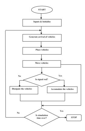
Fig. 1 Overview of the Simulation Framework
