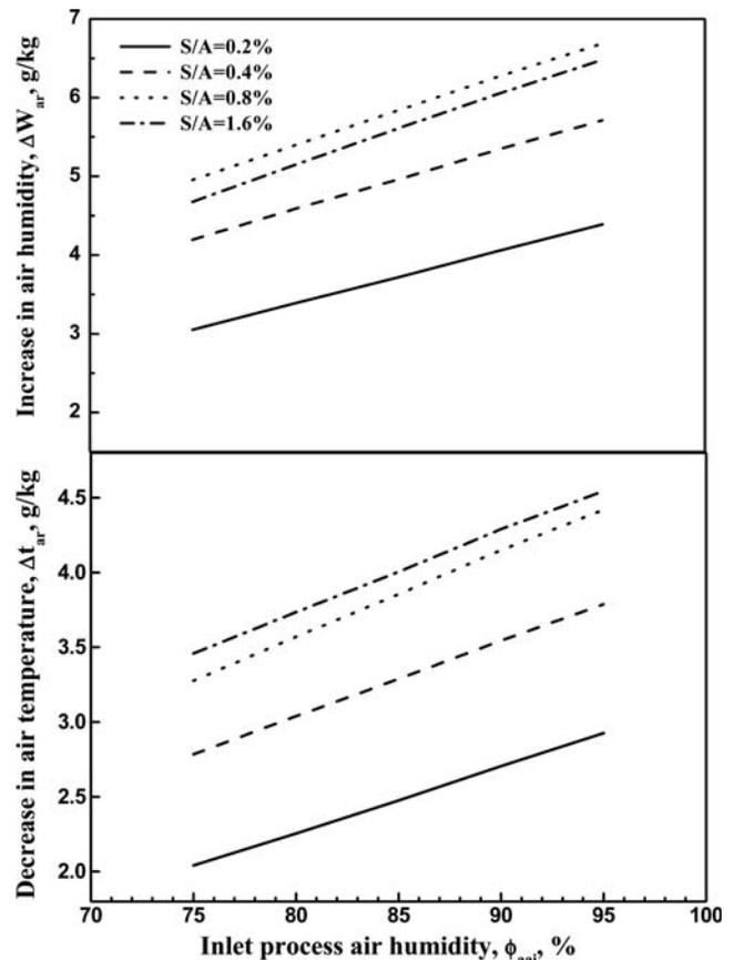
Figure 10. Effect of inlet process air humidity on humidification and cooling of regenerator air in regenerator.
