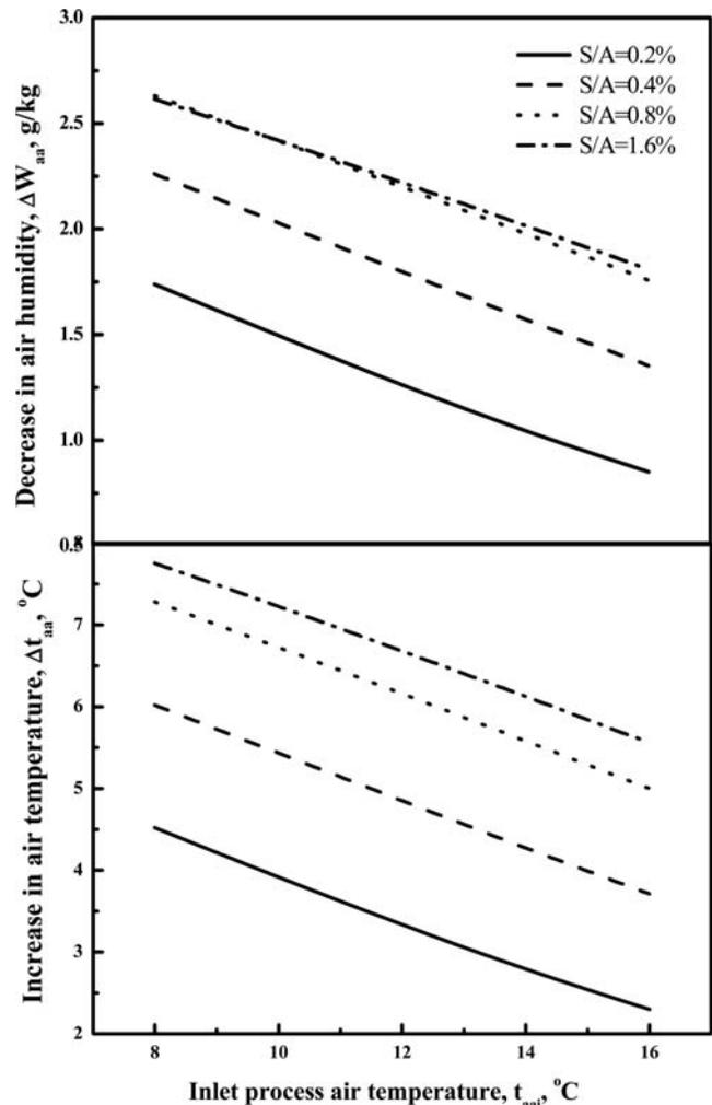
Figure 6. Influence of inlet process temperature on dehumidification and heating of process air in absorber at constant specific humidity.
