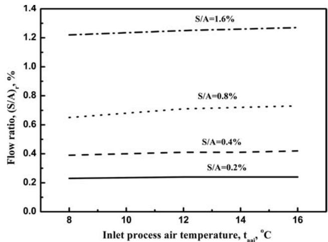
**Figure 4.** Effect of inlet process air temperature on flow ratio in regenerator.
