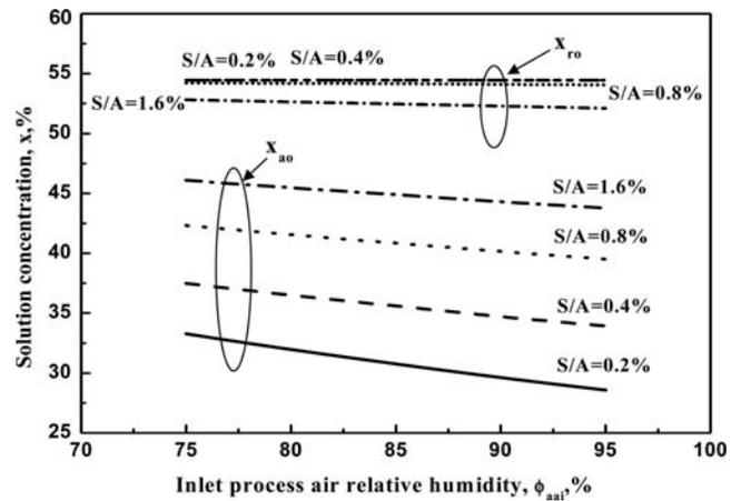
**Figure 3.** Effect of inlet process air relative humidity on solution concentration.
