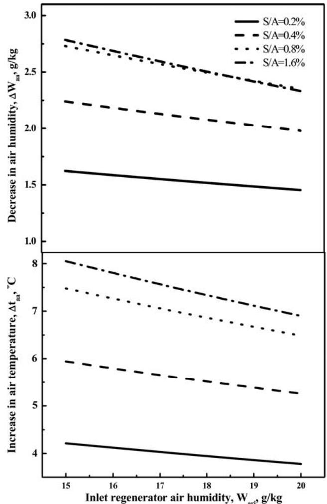
Figure 12. Effect of regenerator air humidity on dehumidification and heating of process air in absorber.
