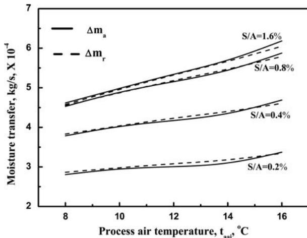
Figure 13. Effect of inlet process air temperature on moisture transfer.
