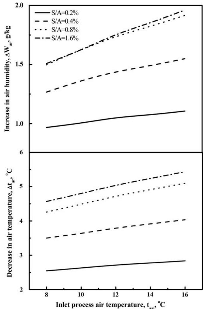
Figure 8. Influence of inlet process air temperature on humidification and cooling of regenerator air in regenerator.
