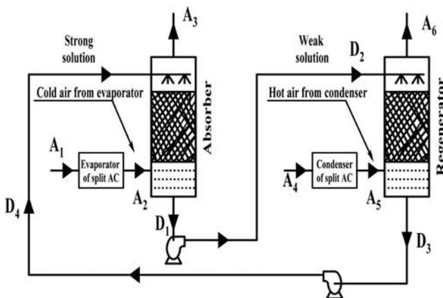
Figure 1. Block diagram of the proposed coupled counter flow columns.
