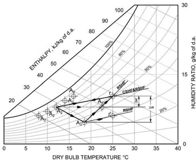
Figure 14. Dehumidification process representation on a psychrometric chart.
