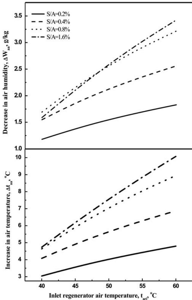
Figure 11. Effect of regenerator air temperature on dehumidification and heating of process air in absorber.
