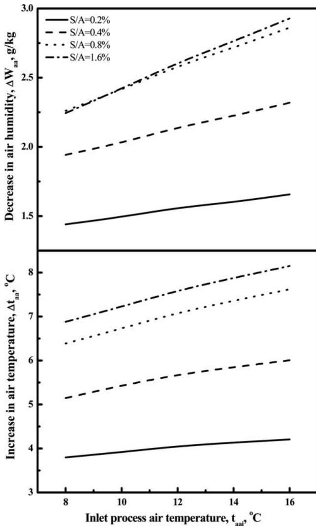
Figure 5. Influence of inlet process temperature on dehumidification and heating of process air in absorber at constant relative humidity.
