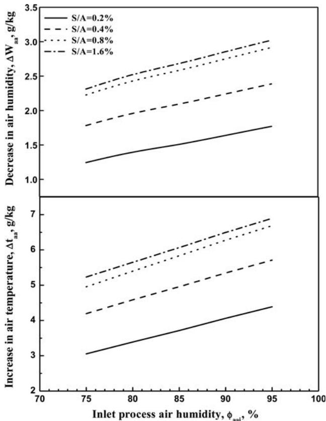
Figure 9. Effect of inlet process air humidity on dehumidification and heating of process air in absorber.
