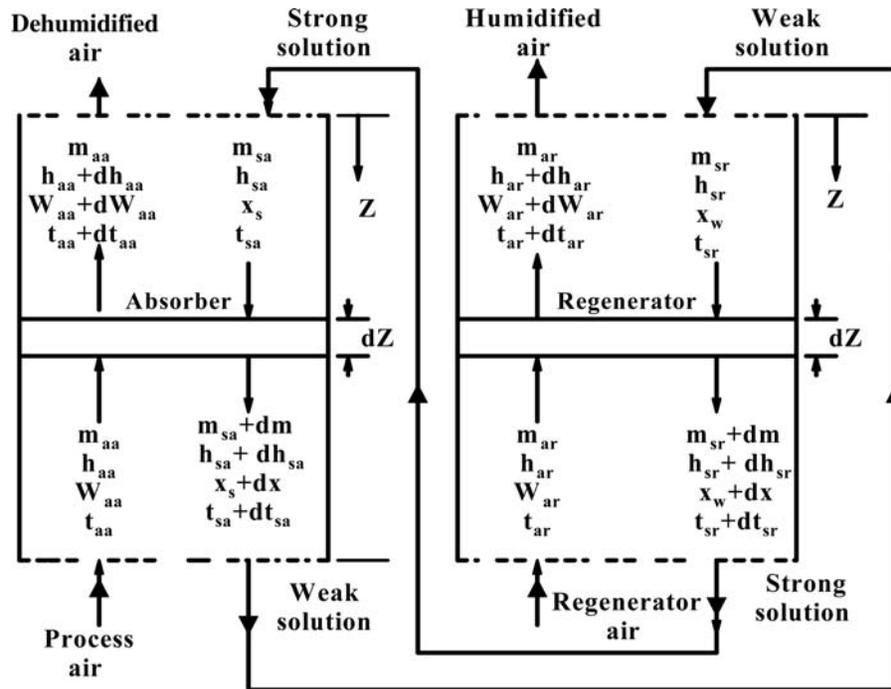
Figure 2. Computational model of the coupled counter flow columns.
