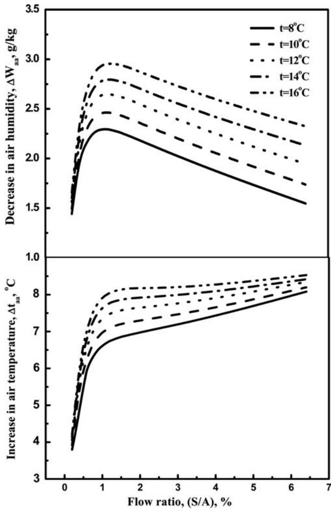
Figure 7. Influence of S/A ratio on dehumidification and heating of process air in absorber at constant relative humidity.
