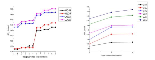
**Figure 3.** SDx values for different TL configurations when  $\Delta \theta = 45^{\circ}$ .
