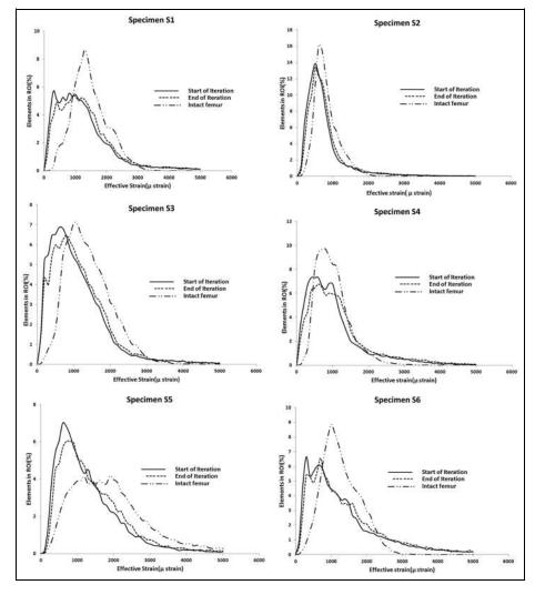
Figure 8. Effective strain histograms in ROI for intact femur bone, bone-implant assembly before and after stiffness optimization in the custom implants.
