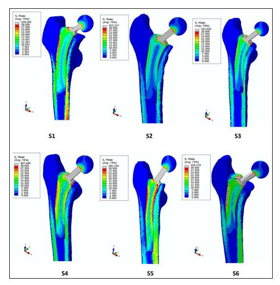
Figure 7. von Mises stresses in implant-bone assembly for the stiffness-optimized custom implants for six femur specimens.
