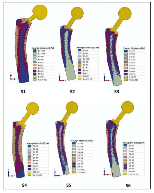
Figure 6. Stiffness-optimized custom implants showing elastic modulus distribution for six femur specimens.
