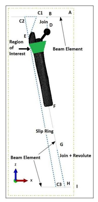
**Figure 2.** FE model of implant-bone assembly with load jig for simulation.
