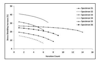
**Figure 5.** Decrease in stress shielding with iterations of numerical optimization of elastic modulus distribution in custom implant.
