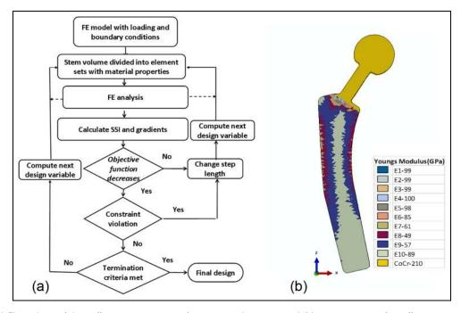
Figure 4. (a) Flow chart of the stiffness optimization of custom implant stem and (b) cross section of a stiffness-optimized implant with elastic modulus distribution.
