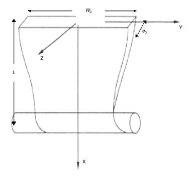
Fig. 1.1. Sketch of the geometry considered for the film casting process.
