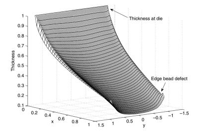
Fig. 1.2. Thickness profile of the film casting process with edge bead defect.
